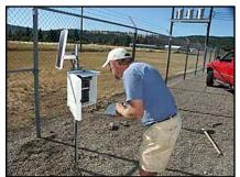
Researchers have installed four climate stations around the watershed to monitor precipitation, wind, solar radiation, temperature, and soil moisture conditions that will enable better estimates of infiltration versus evapotranspiration rates regionally. Ultimately these values will replace theoretically-derived values initially used which will reduce uncertainty in the model and thus improve management decisions.
