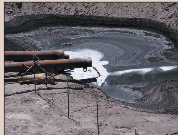
Figure 27 · Liquid hydrocarbons and product water may be discharged to the surface during the drilling phase of CBM development.
